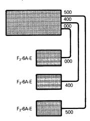
The analog input/output unit may be used up to a maximum of three units, depending upon the type name of basic unit used for the programmable controller.
