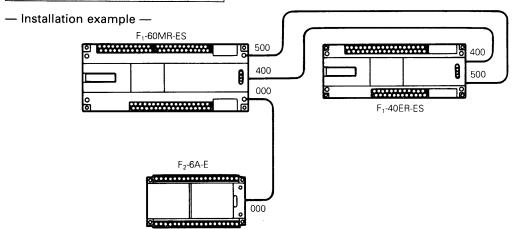
The extension unit may be installed at the upper side/lower side or the right-hand side of the basic unit.
