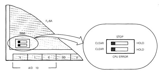
**Note**: Keep in mind that the mode selection at the CPU ERROR side is treated preferentially over the mode selection at the STOP side.
