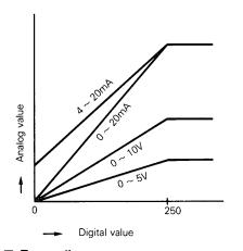
To facilitate the digital/analog conversion, the digital value of 0  $\sim$  250 is generally converted into the analog value of 0  $\sim$  5V, 0  $\sim$  10V, 0  $\sim$  20mA, 4  $\sim$  20mA, etc.
