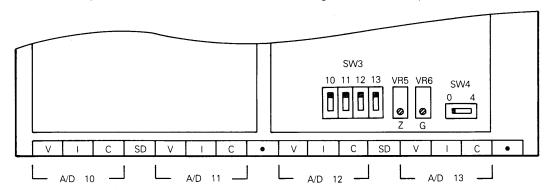
To set the input type, change SW3 and SW4 as shown in the following table;
