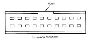
The extension unit is most readily affected by noise, therefore, be sure to keep it away from the other electrical wirings more than  $30 \sim 50$ mm.
