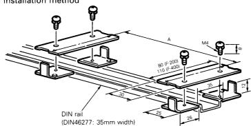
Do not attempt to install the unit on the floor or ceiling, but on the wall surface, for prevention of temperature rise.
